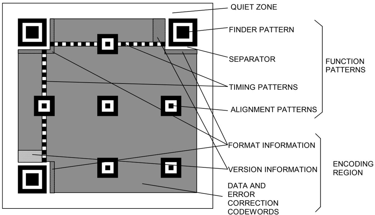
**Figure 3 — Structure of a QR Code 2005 symbol**
