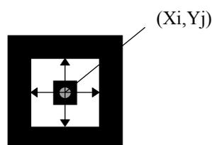
Figure 35 — Central coordinates of alignment pattern
