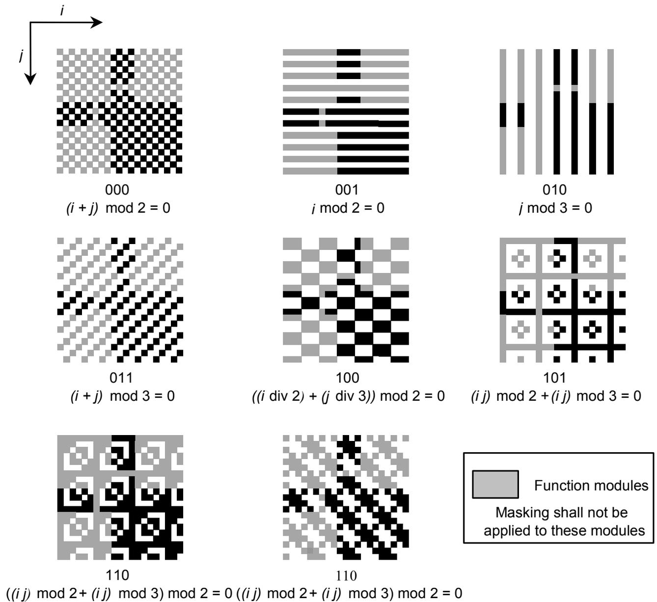
Figure 21 — Data mask patterns for version 1 symbol
