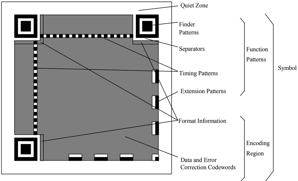
Figure N.1 — Structure of a QR Code Model 1 symbol
