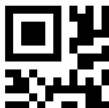
**Figure I.4 — Final version M2-L symbol encoding 01234567**
