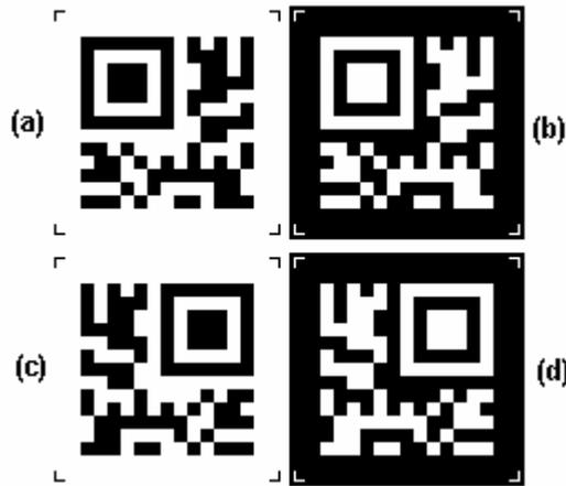
**Figure 2 — Examples of Version M2 Micro QR Code symbol encoding the text "01234567" – (a) normal orientation and normal reflectance arrangement; (b) normal orientation and reversed reflectances; (c) mirror image orientation and normal reflectance arrangement; (d) mirror image orientation and reversed reflectances**
