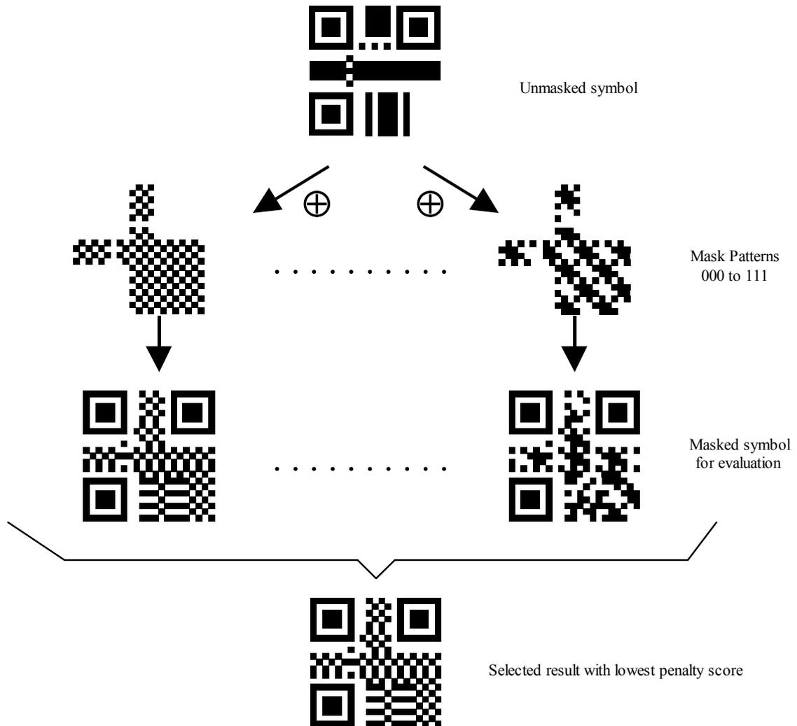
Figure 23 — Data masking simulation in QR Code symbols
